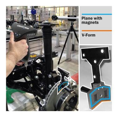
Automatic alignment drastically reduces measurement times and eliminates major sources of errors. For example, an inline inspection system was installed by Creaform at Aircelle (Safran Group) to verify the inline of an aircraft's reverser doors. The inspection time was reduced by three and the number of errors by more than five compared with a mechanical portable CMM.
